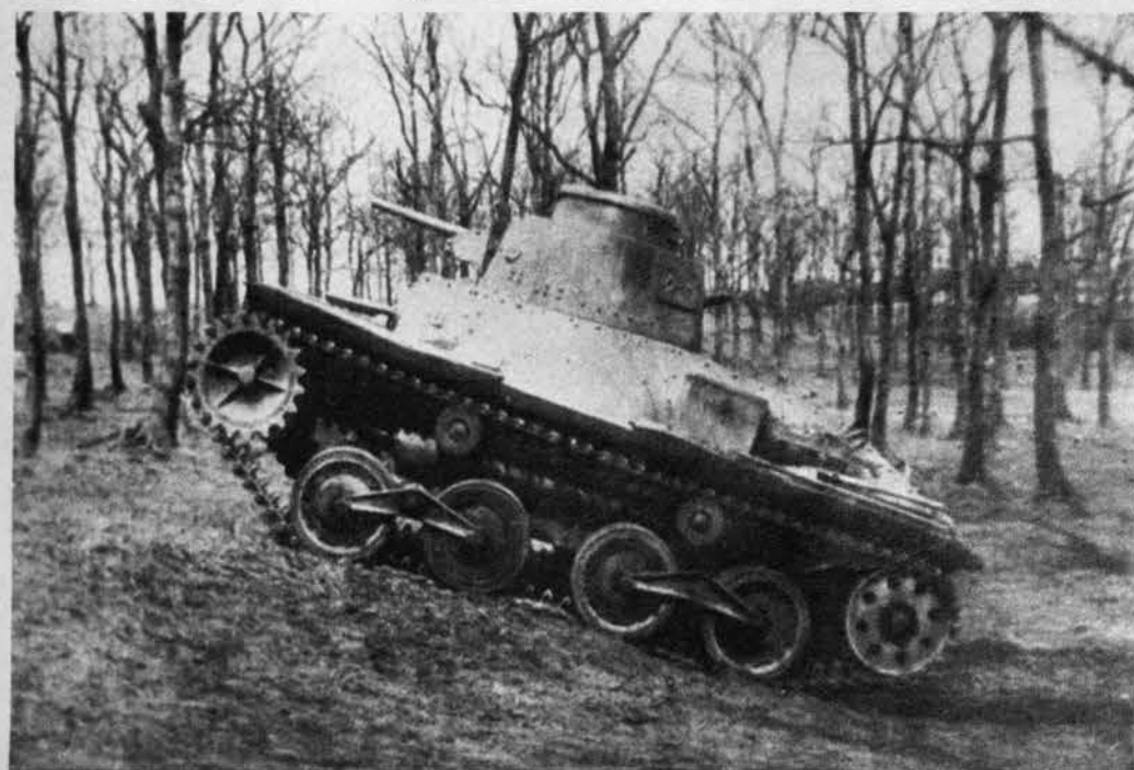
Basic Jap suspension system consists of bell-crank arms holding a rocking pair of bogie wheels. The light tank 2595 shown here, built in 1935, has two pairs of bogie wheels and two return rollers supporting a narrow track, with the driving sprocket in front. Its top speed is 25 to 30 m.p.h.
